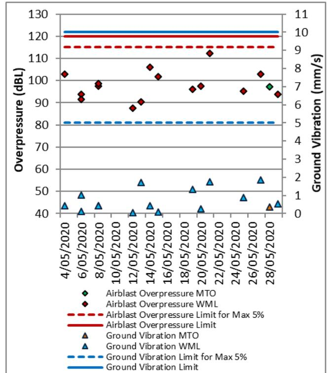
Figure 13: Wambo Road Blast Monitoring Results – May 2020
