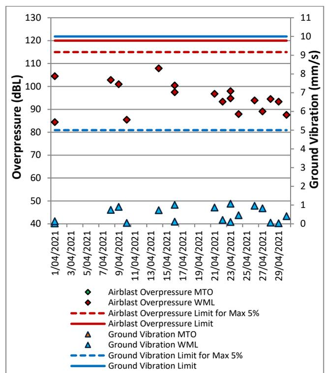
Figure 13: Wambo Road Blast Monitoring Results – April 2021
