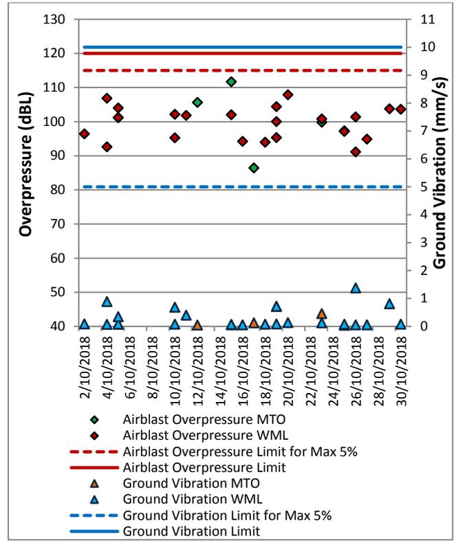
Figure 13: Wambo Road Blast Monitoring Results – October
