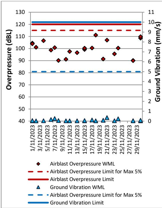
Figure 11: MTIE Blast Monitoring Results – November 2023
