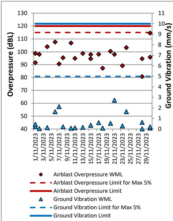
Figure 12: Wollemi Peak Road Blast Monitoring Results – November 2023
