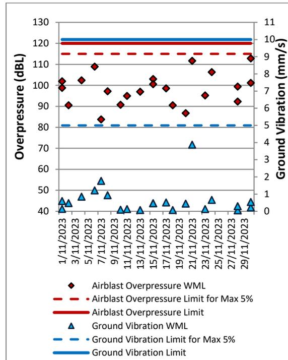
Figure 14: Warkworth Blast Monitoring Results – November 2023
