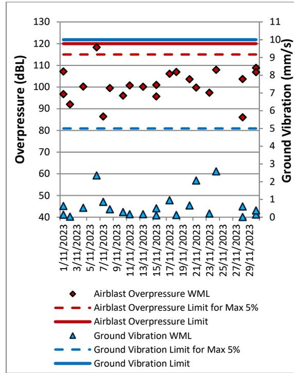
Figure 13: Wambo Road Blast Monitoring Results – November 2023
