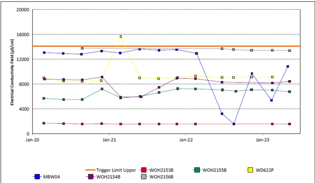
Figure 34: Wambo Seam Electrical Conductivity Field Trend – June 2023
