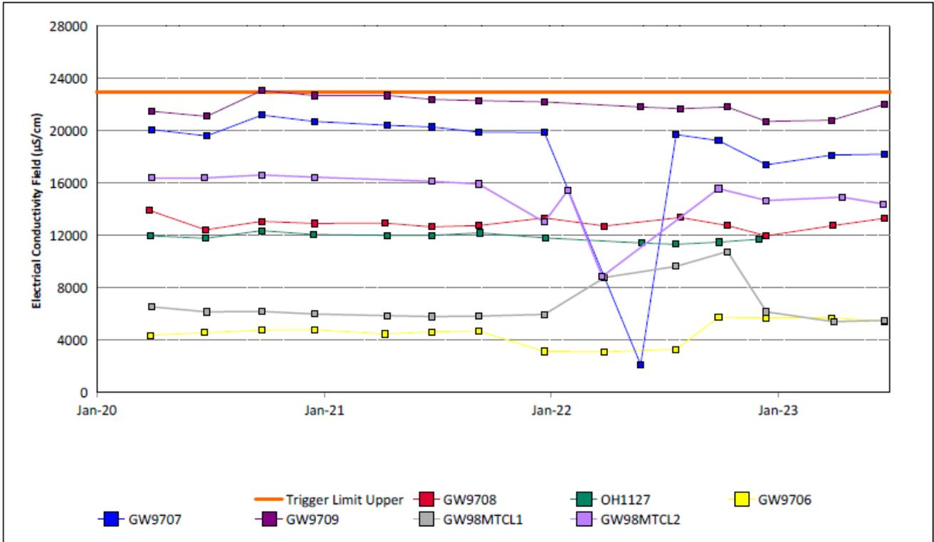
Figure 16: Bayswater Seam Electrical Conductivity Field Trend – June 2023
