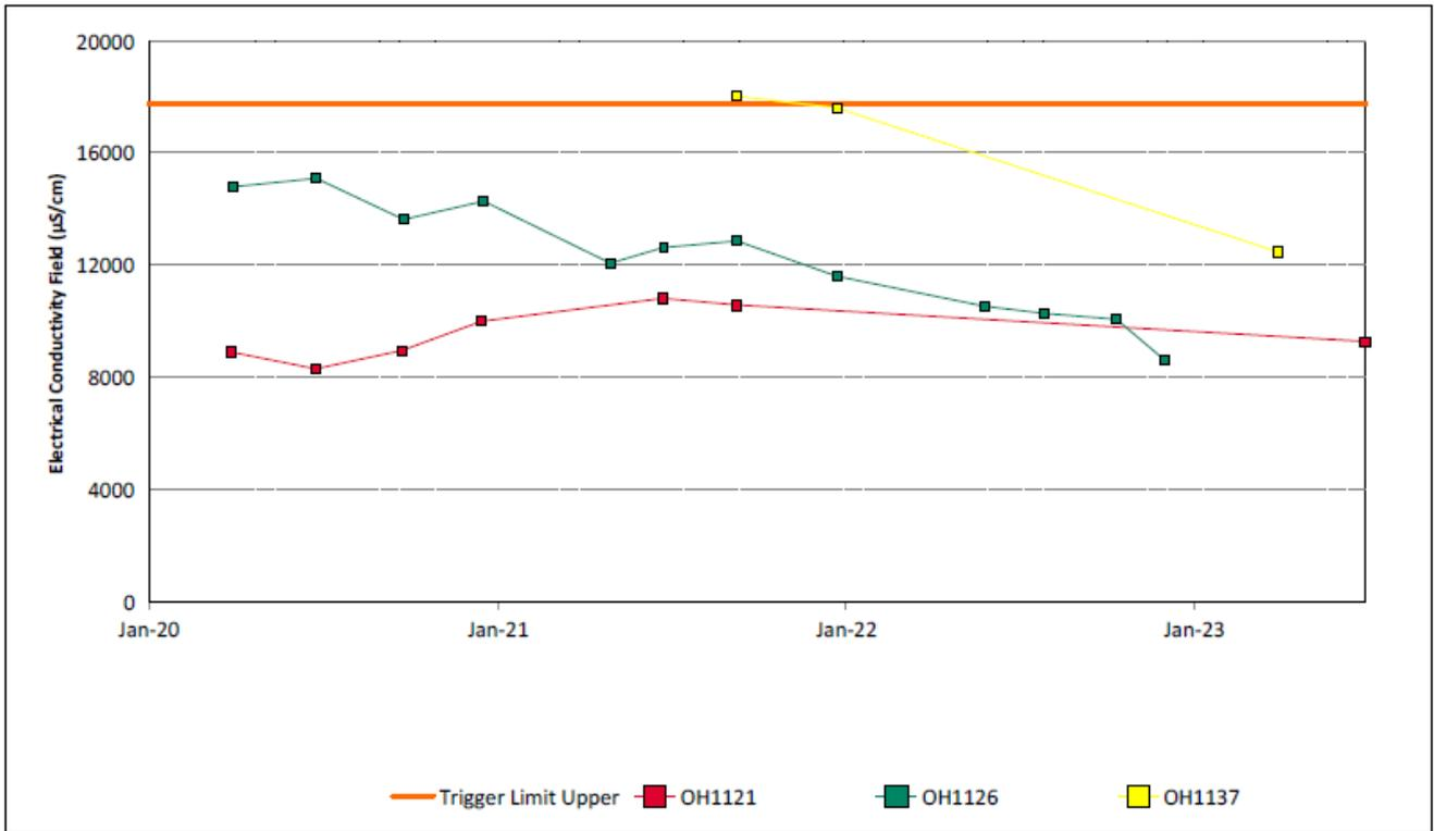
Figure 31: Vaux Seam Electrical Conductivity Field Trend – June 2023
