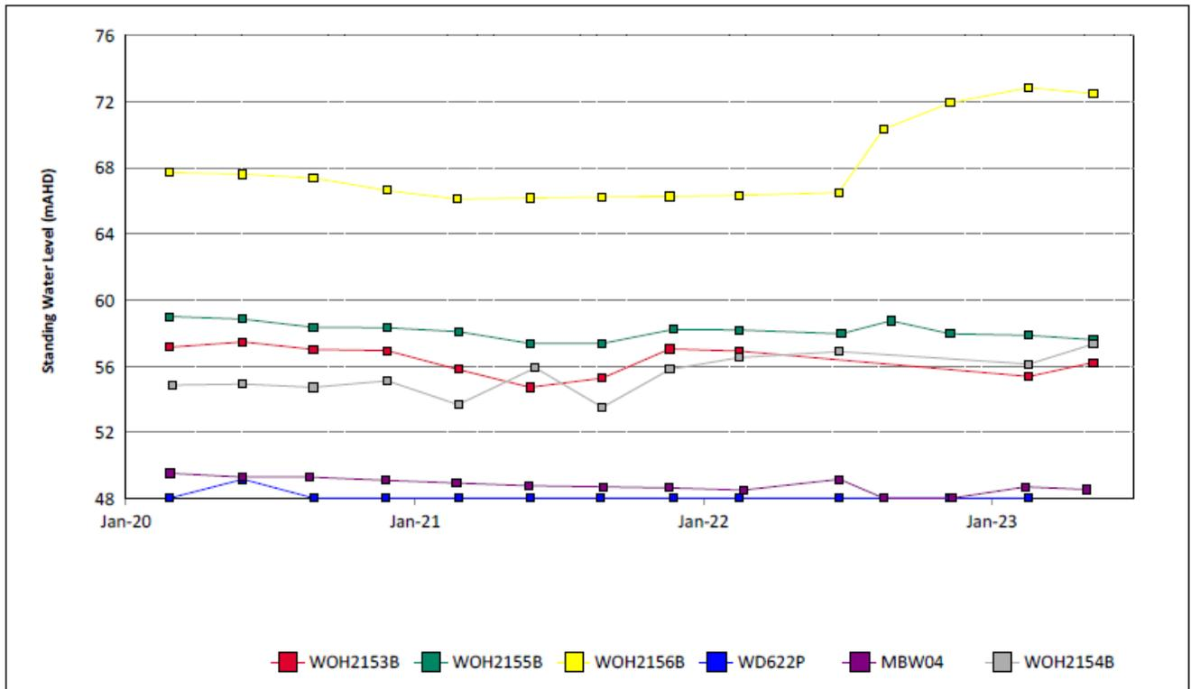
Figure 36: Wambo Seam Standing Water Level Trend – June 2023
