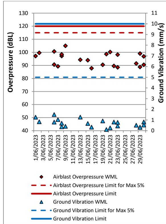
Figure 70: Warkworth Blast Monitoring Results – June 2023
