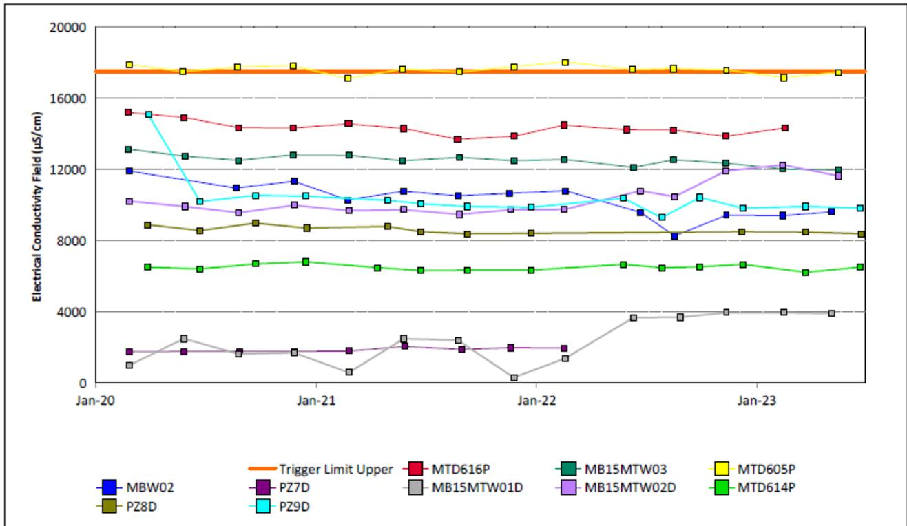
Figure 28: Shallow Overburden Electrical Conductivity Field Trend – June 2023
