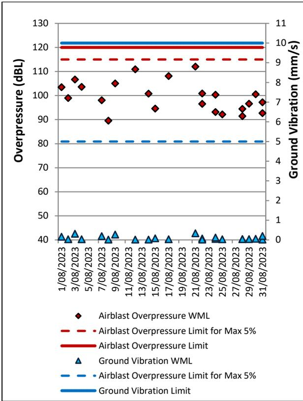
Figure 11: MTIE Blast Monitoring Results – August 2023
