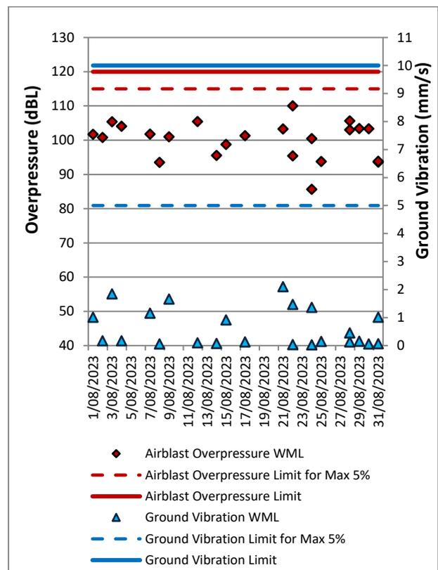
**Figure 10: Bulga Village Blast Monitoring Results – August 2023**
