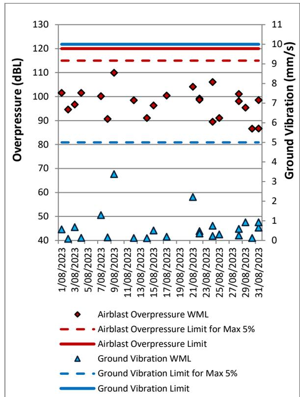
Figure 14: Warkworth Blast Monitoring Results – August 2023
