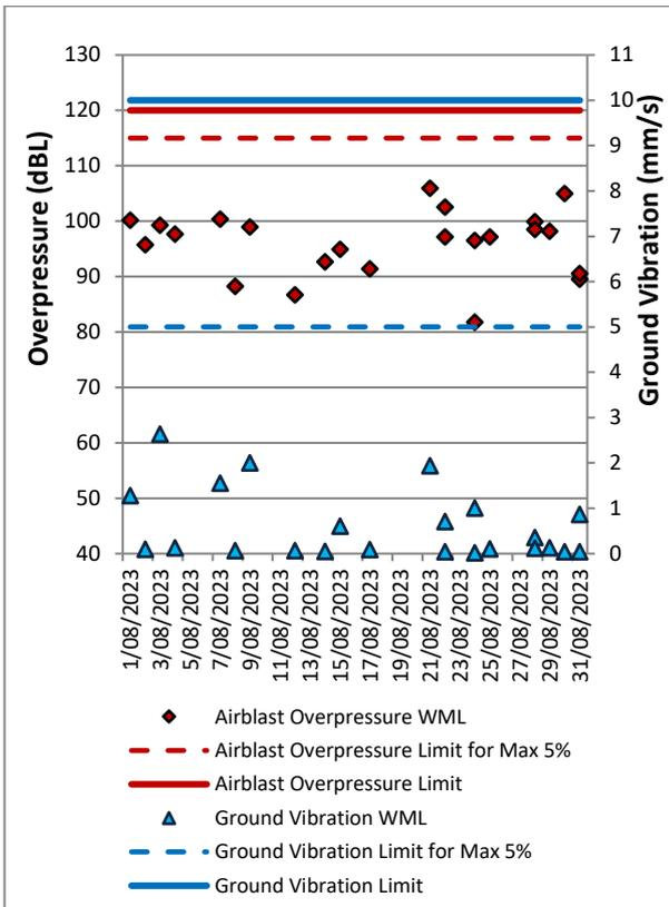
Figure 12: Wollemi Peak Road Blast Monitoring Results – August 2023
