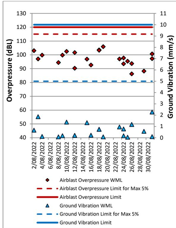
Figure 13: Wambo Road Blast Monitoring Results – August 2022
