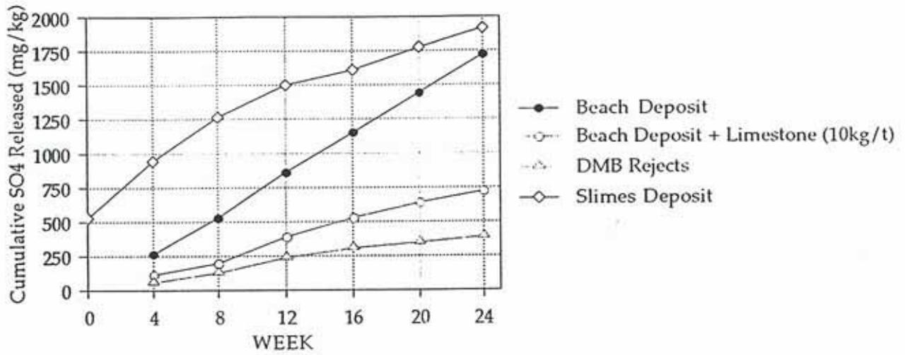
Figure 10: Cumulative SO<sub>4</sub> release with leaching.
