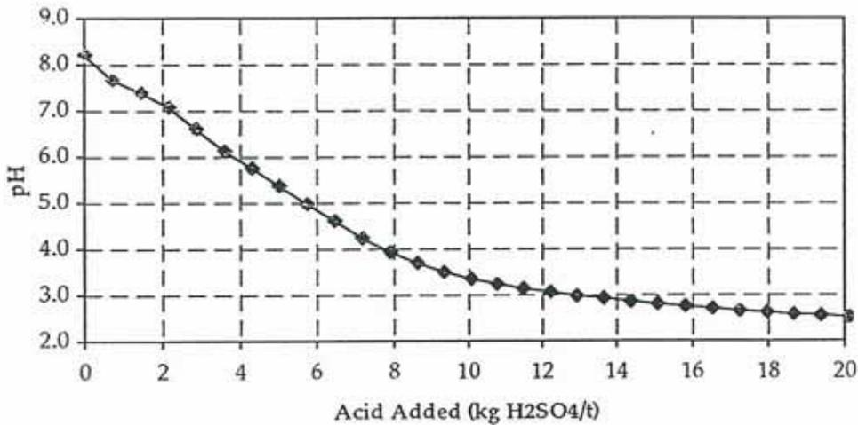
Figure 2: Acid buffering characteristic curve for Co-Disposed Beach Deposit sample CDB2 with a measured ANC of 32 kg H<sub>2</sub>SO<sub>4</sub>/t.
