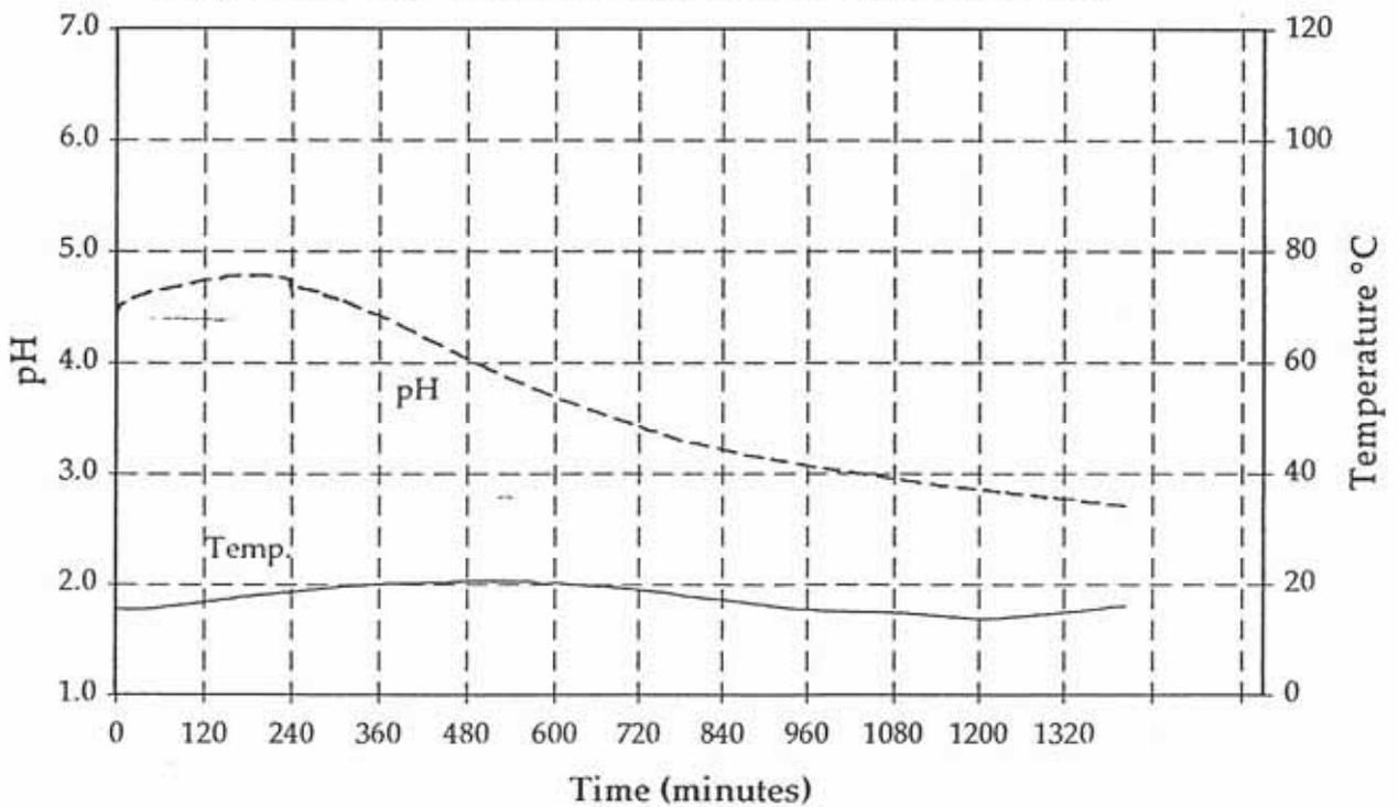
Figure 3: Kinetic NAG Profile for Co-disposed Slime (CDS3).
