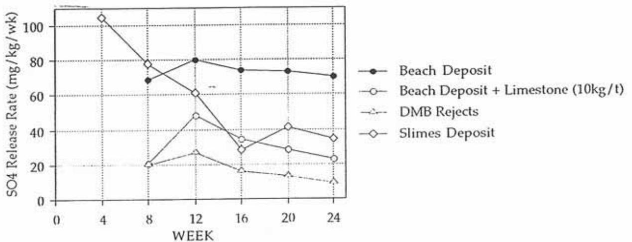
Figure 9: Sulphate release rate trend with leaching.
