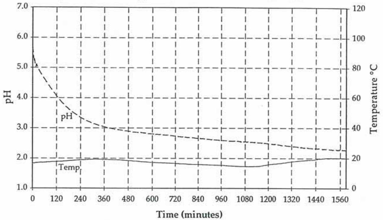
Figure 2: Kinetic NAG Profile for DMB-reject (DMB2).
