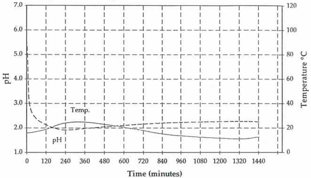
Figure 4: Kinetic NAG Profile for Co-disposed Beach Deposit (CDB2).
