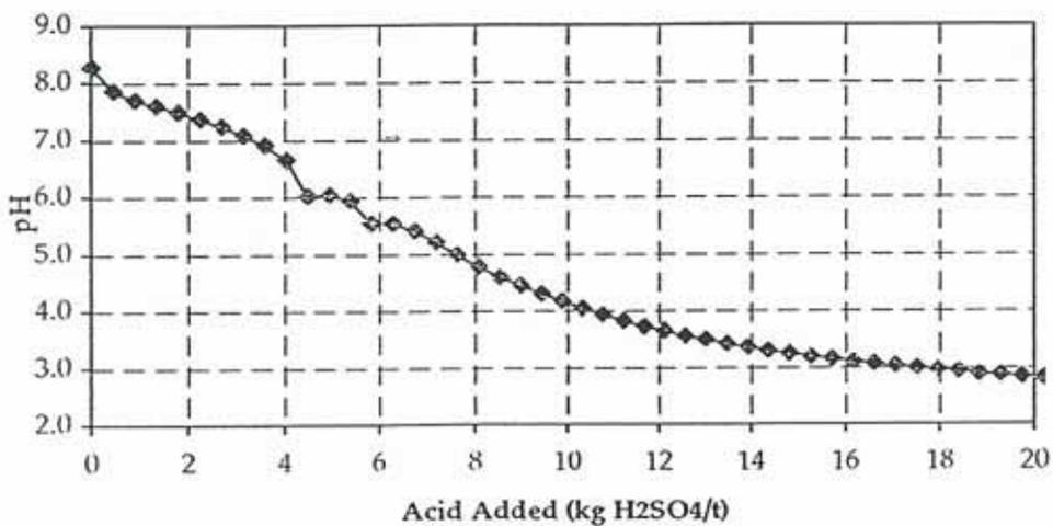
Figure 3: Acid buffering characteristic curve for Co-Disposed Slimes sample CDS1 with a measured ANC of 15 kg H<sub>2</sub>SO<sub>4</sub>/t.
