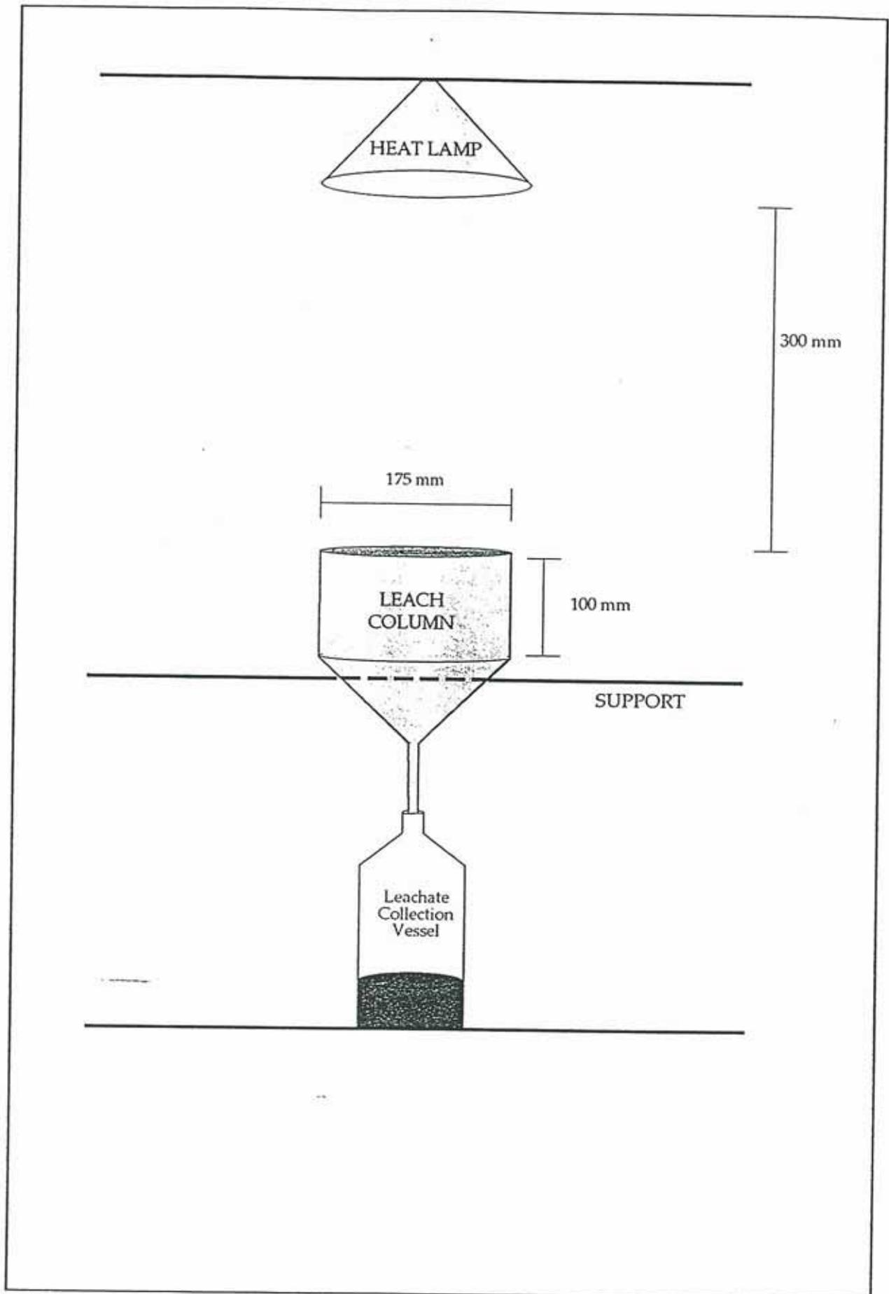
Figure A1: Schematic diagram of leach column set-up.
