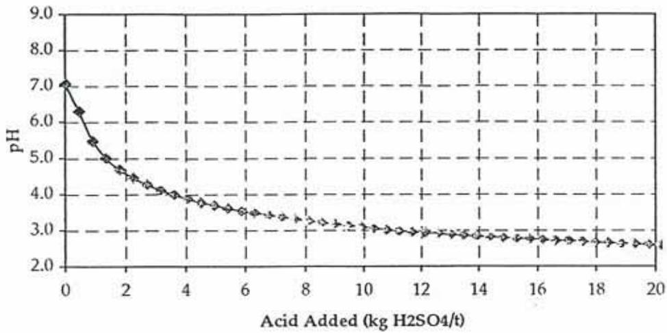
Figure 1: Acid buffering characteristic curve for DMB Rejects Composite sample (DMB2 & DMB 3) with a calculated ANC of 17 kg H<sub>2</sub>SO<sub>4</sub>/t.
