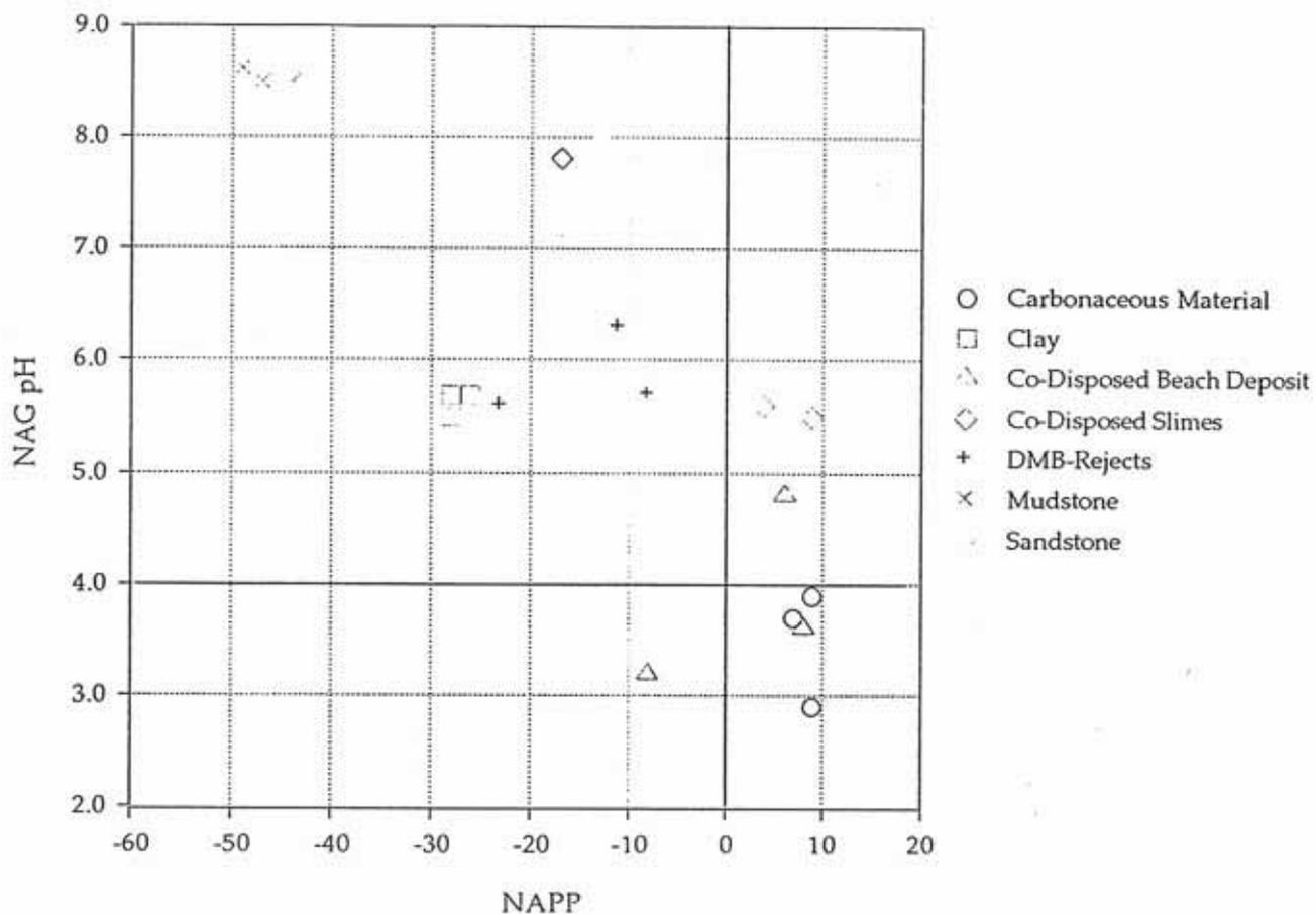
Figure 1: NAPP vs NAGpH for Stratford Coal Reject and Spoil Samples - Split by Material Type
