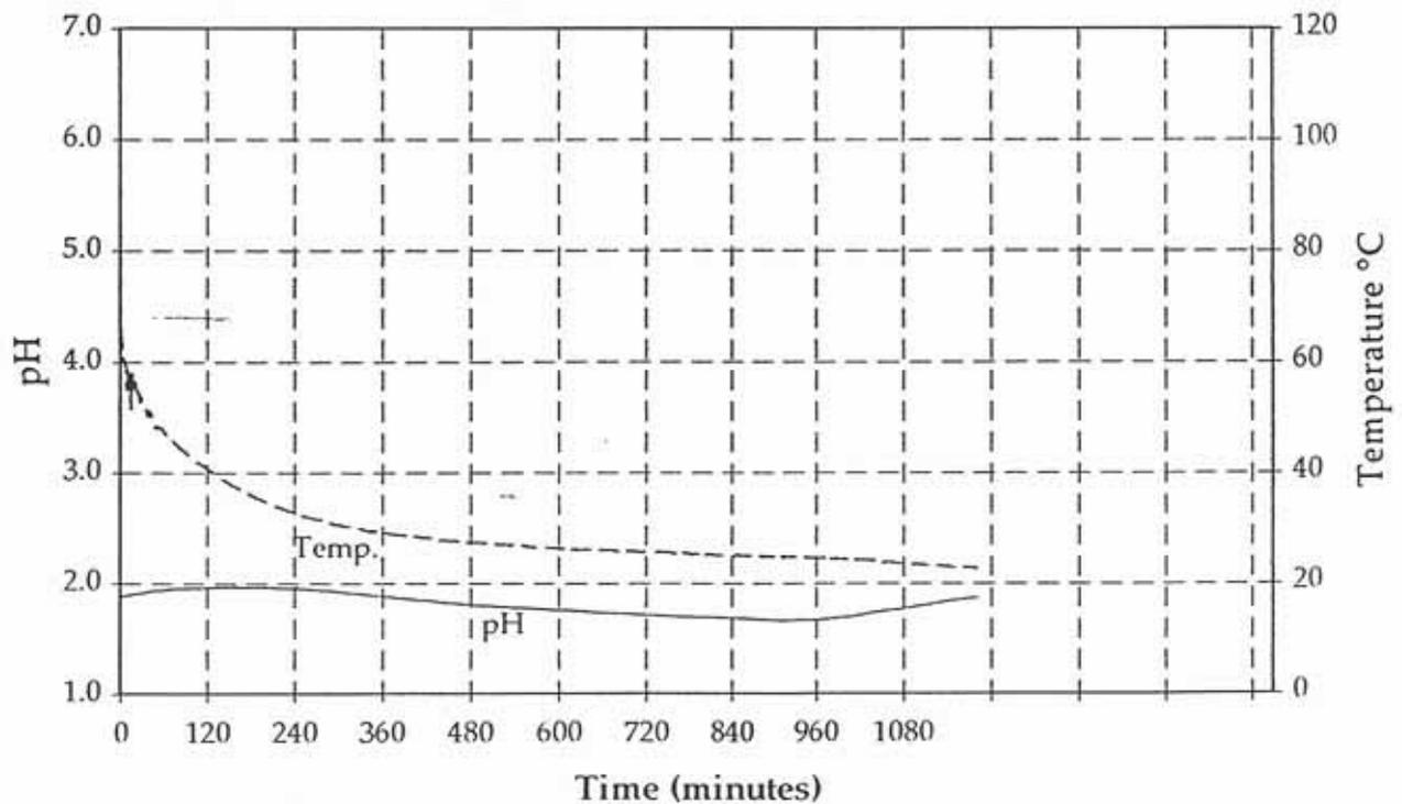
Figure 5: Kinetic NAG Profile for Carbonaceous Material (CM1).
