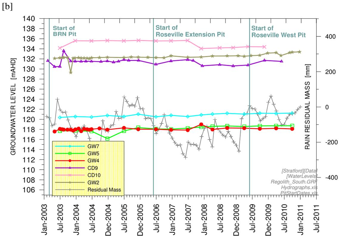
Figure A-18 Groundwater Hydrographs in Regolith: [a] north; [b] south
