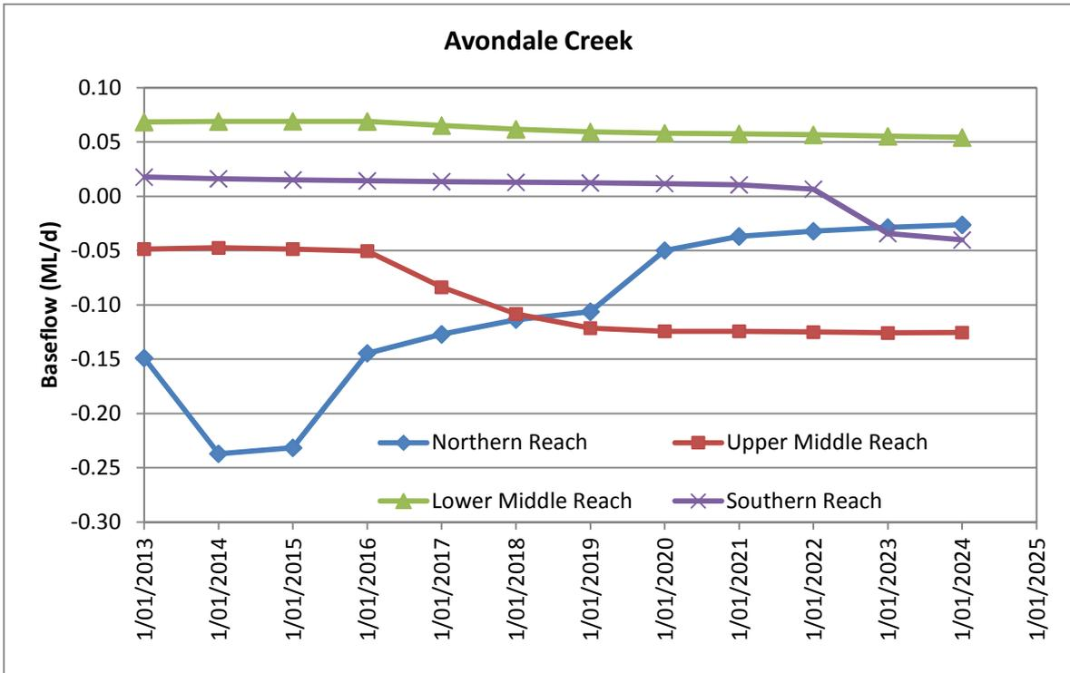
Figure A-51. Simulated Changes in Baseflow to Avondale Creek Reaches during the Project
