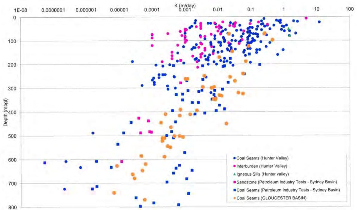
Figure A-34. Comparative Hydraulic Conductivity Measurements in the Gloucester Basin, Sydney Basin and Hunter Valley [Source: Tammetta, 2009]
