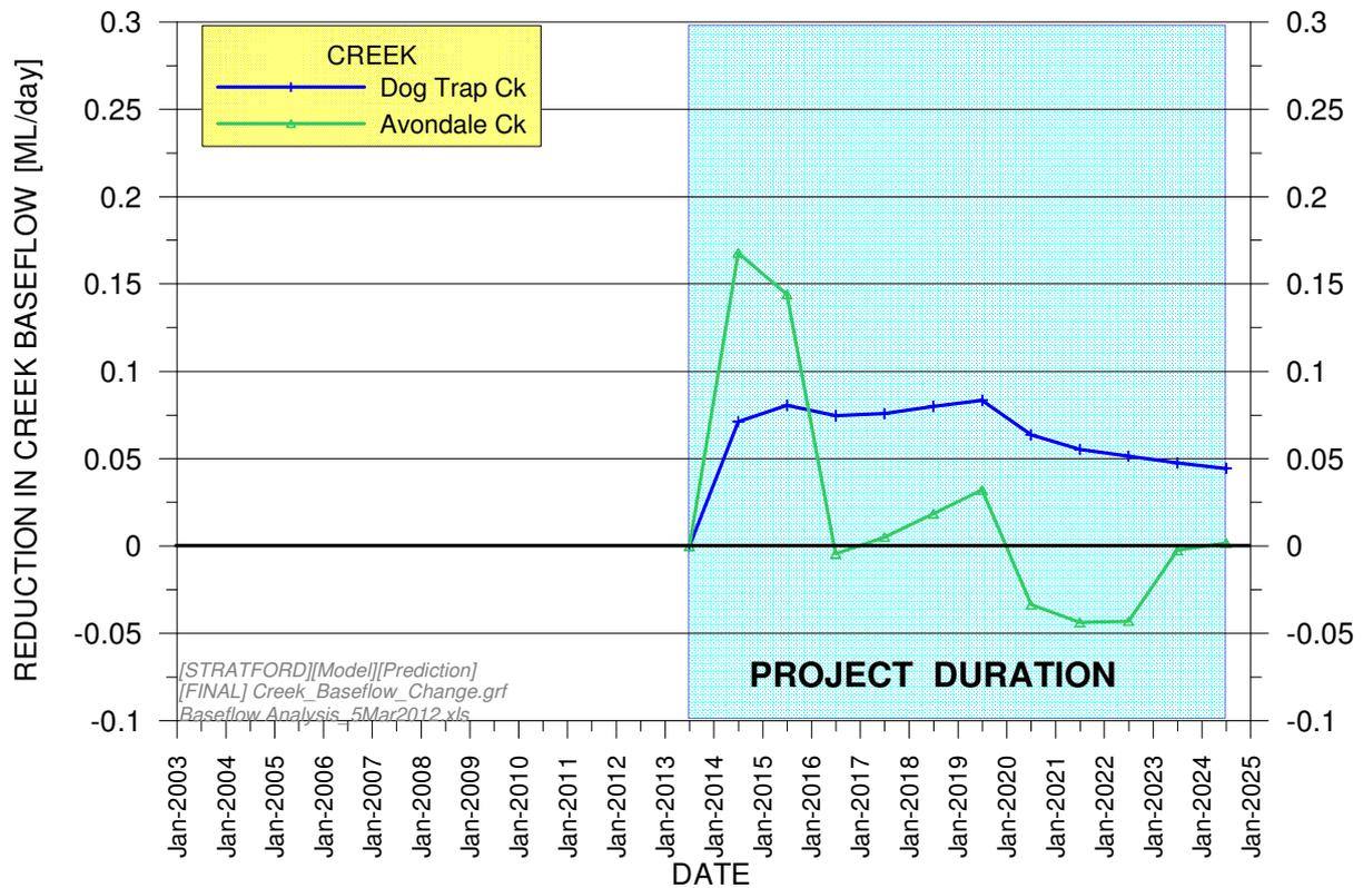
Figure A-50. Simulated Reduction in Baseflow to Dog Trap Creek and Avondale Creek during the Project
