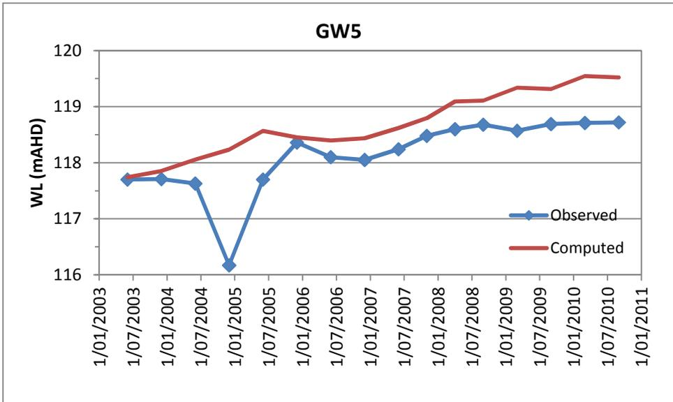
Figure A-44. Representative Simulated and Measured Hydrographs at Bores Screened in Regolith [MW9 and GW5]
