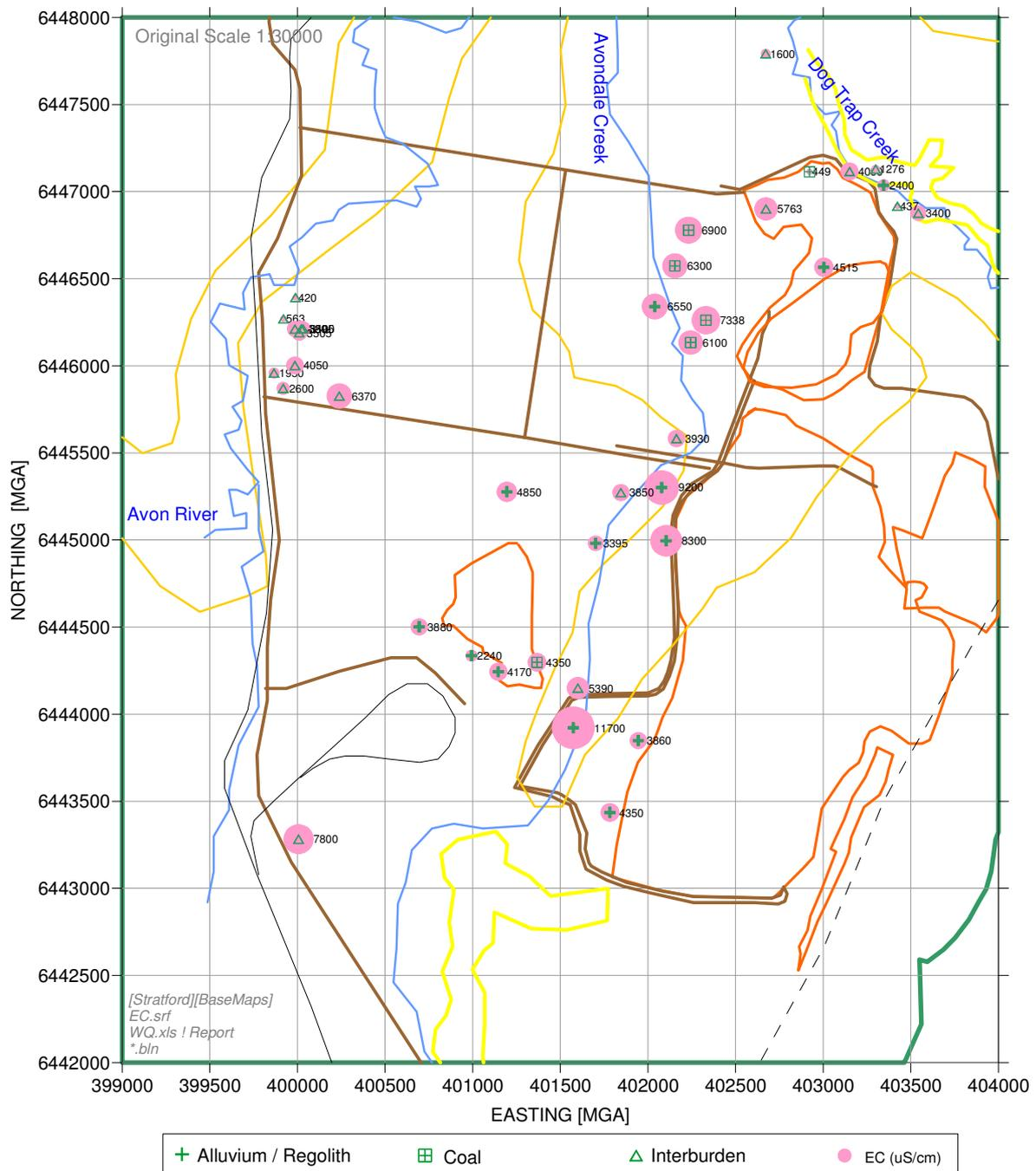
Figure A-24 Spatial Distribution of Groundwater Electrical Conductivity [ $\mu\text{S}/\text{cm}$ ]
