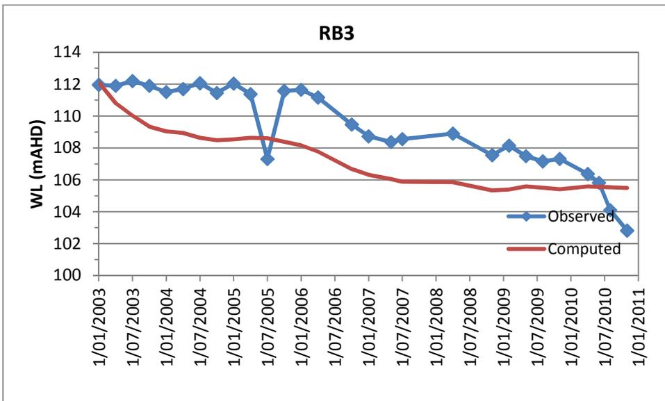
Figure A-45. Representative Simulated and Measured Hydrographs at Bores Screened in Interburden [MW5 and RB3]
