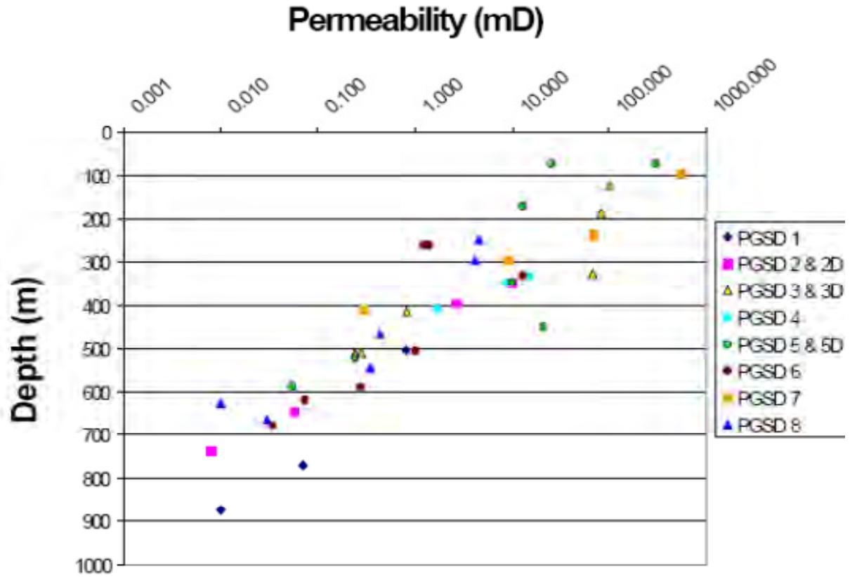
Figure A-33. Intrinsic Permeability Measurements of Coal Seams at Stratford in the Gloucester Basin [Source: Smith, 2001]
