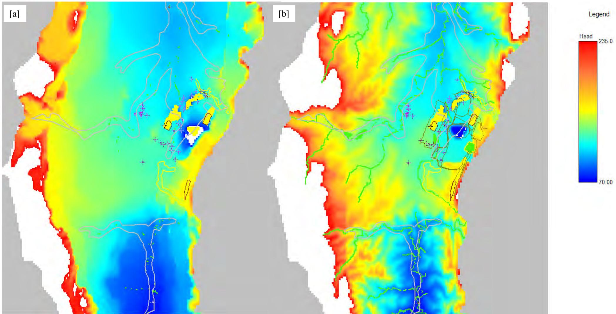
Figure A-38. Simulated Layer 1 Watertable Elevations at [a] Steady State; [b] End of Transient Calibration Period (June 2010) [mASD]
