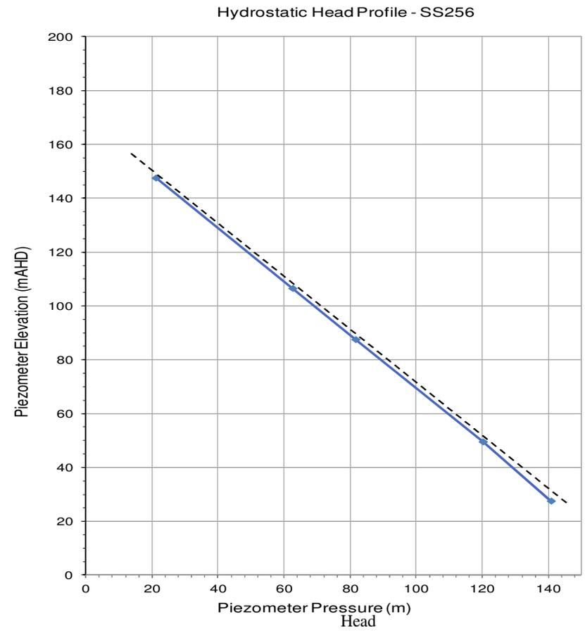
Figure A-15 Multi-level Vibrating Wire Groundwater Piezometer Hydrostatic Plots for GC207 and SS256
