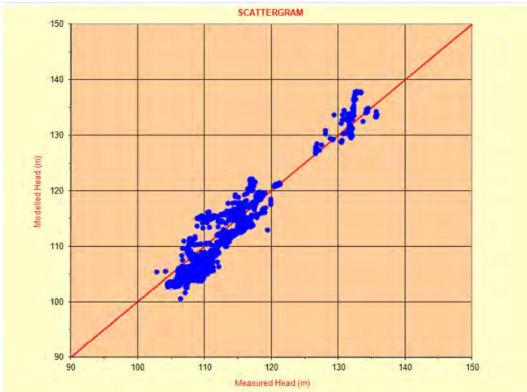
Figure A-42. Scattergram of Simulated and Measured Heads for Transient Calibration
