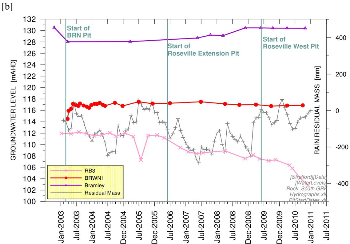
Figure A-19 Groundwater Hydrographs in Interburden: [a] north; [b] south
