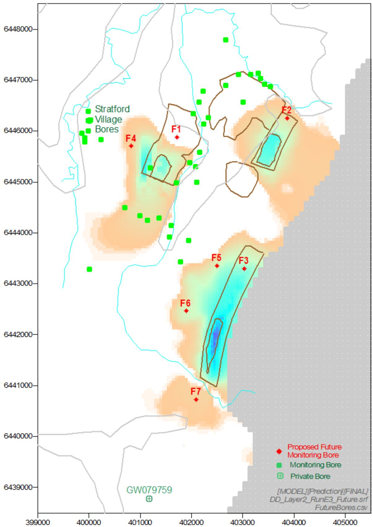
Figure A-60. Proposed Expansion of the Groundwater Monitoring Network
