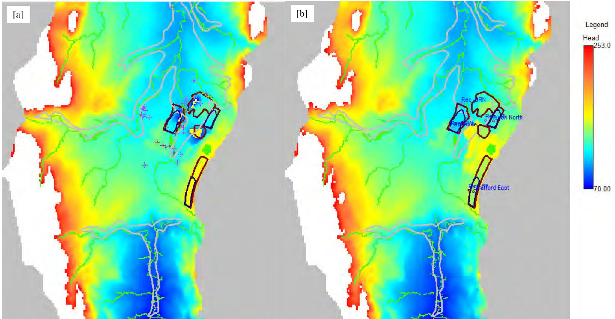
Figure A-56. Simulated Layer 1 Watertable Elevations at [a] End of Transient Calibration Period (June 2010); [b] Post-Mining Final Equilibrium [mAHD]
