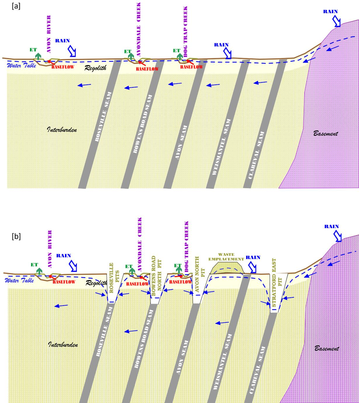
Figure A-25 Conceptual Groundwater Models [a] Natural conditions; [b] During mining.
