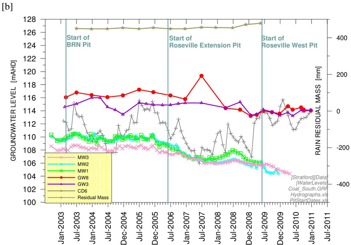
Figure A-17 Groundwater Hydrographs in Coal Seams: [a] north; [b] south
