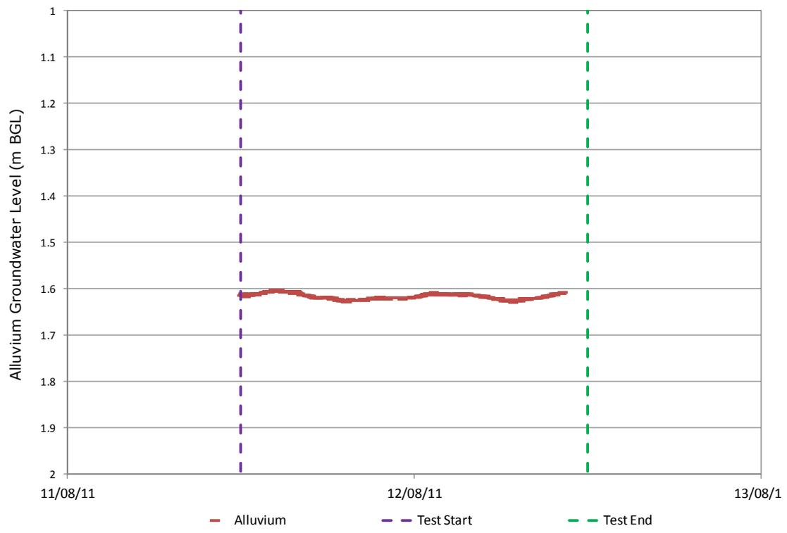
Figure A-27 Pumping Test Restart at Dog Trap Creek (Source RPS Aquaterra, 2011)
