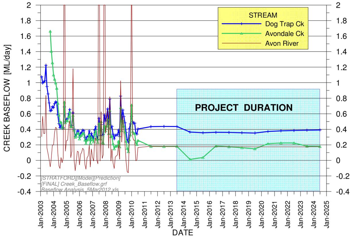
Figure A-49. Simulated Stream-Aquifer Exchanges for Dog Trap Creek, Avondale Creek and Avon River
