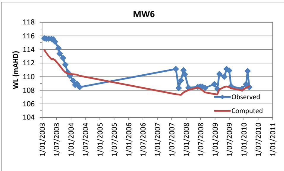
Figure A-43. Representative Simulated and Measured Hydrographs at Bores Screened in Coal [MW1 and MW6]
