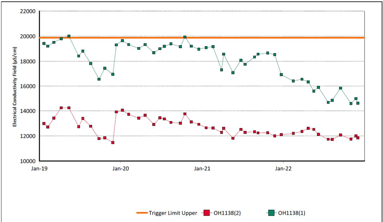
Figure 37: Warkworth Seam Electrical Conductivity Field Trend - December 2022
