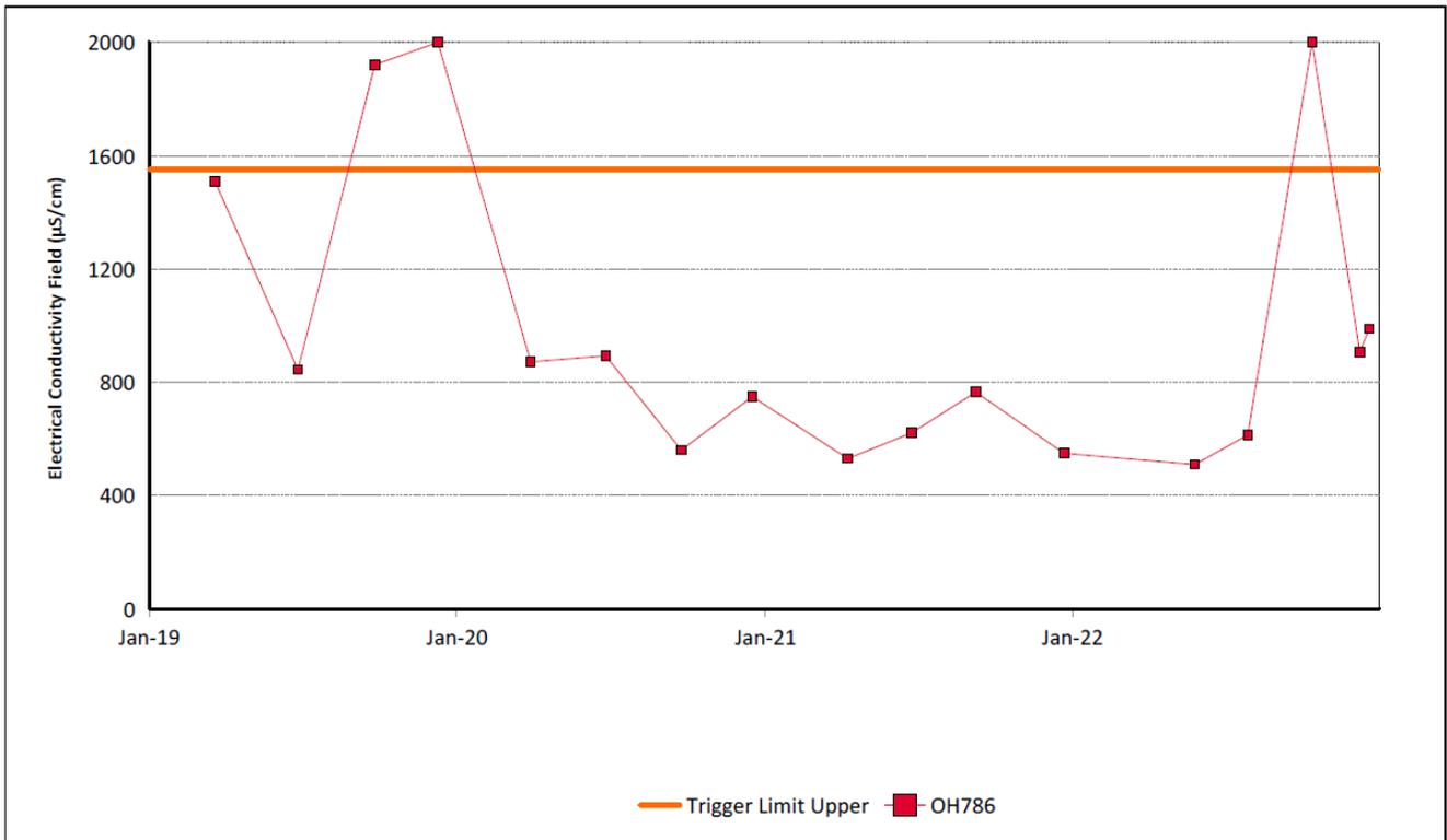
Figure 51: Hunter River Alluvium 1 Electrical Conductivity Field Trend - December 2022
