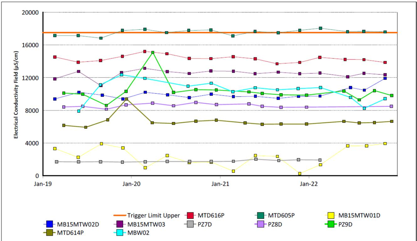
Figure 28: Shallow Overburden Electrical Conductivity Field Trend - December 2022
