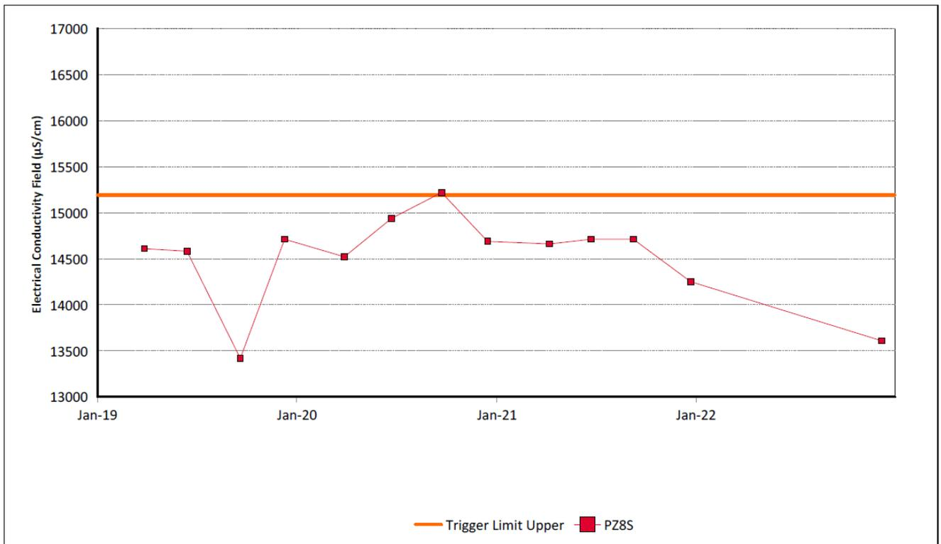
Figure 40: Wollombi Alluvium 1 Electrical Conductivity Field Trend - December 2022
