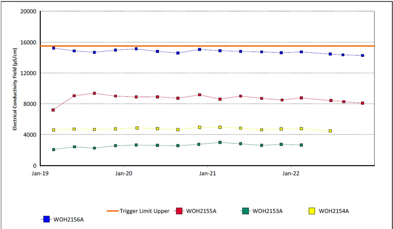
Figure 25: Redbank Seam Electrical Conductivity Field Trend - December 2022
