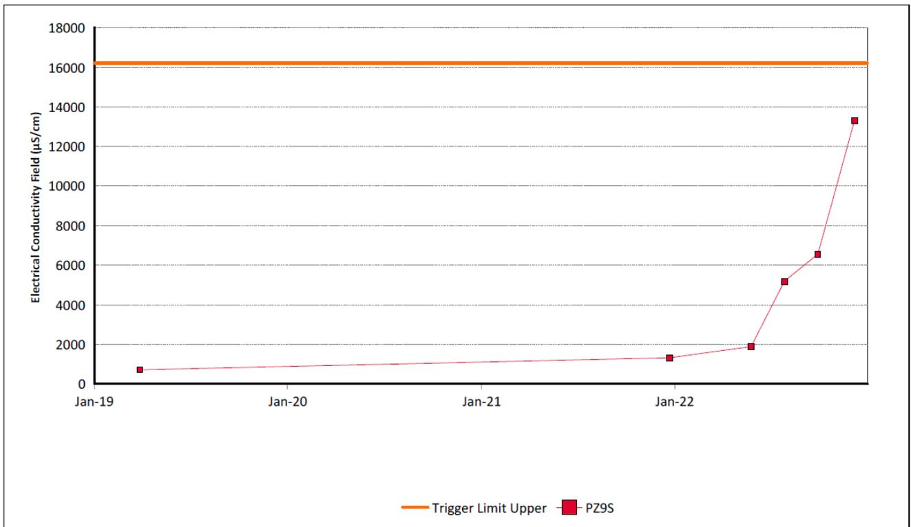
Figure 42: Wollombi Alluvium 2 Electrical Conductivity Field Trend – December 2022
