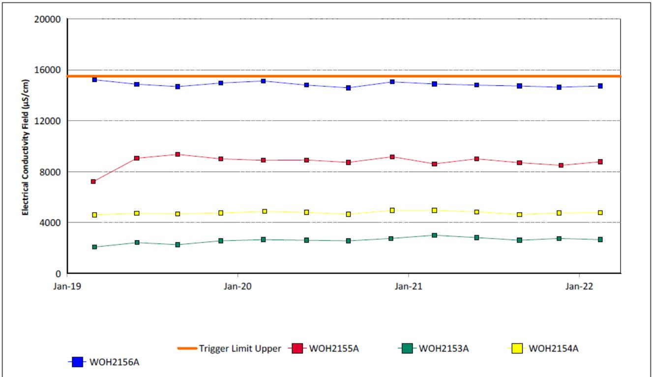
Figure 25: Redbank Seam Electrical Conductivity Trend – March 2022
