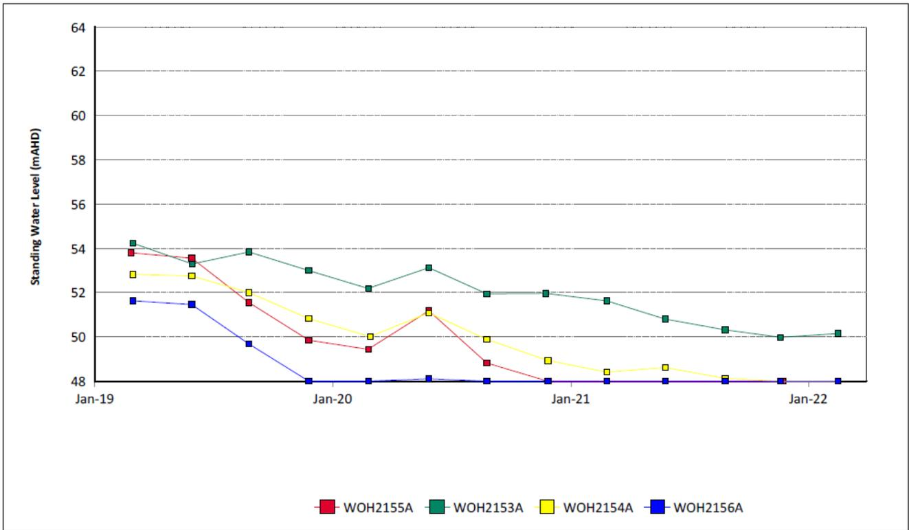
Figure 27: Redbank Seam Standing Water Level Trend – March 2022
