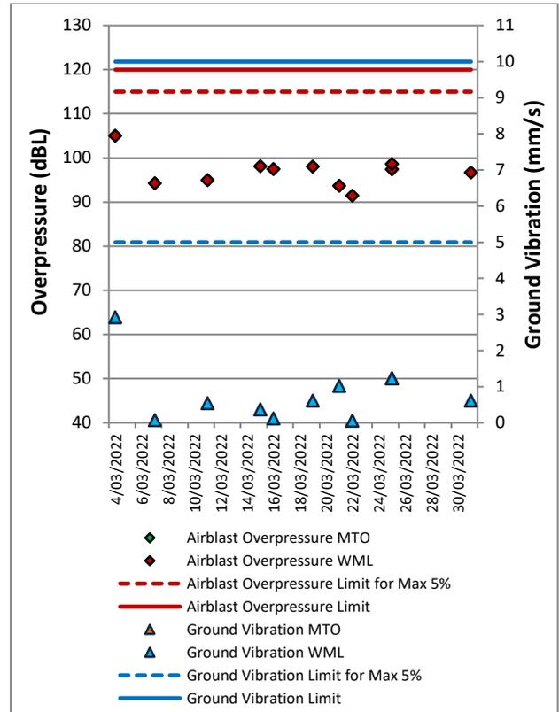
Figure 70: Wambo Road Blast Monitoring Results – March 2022
