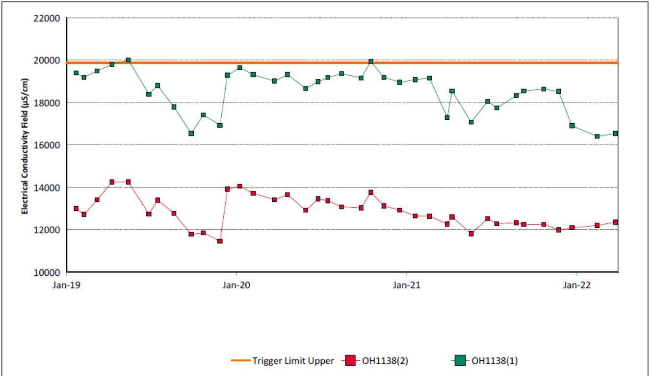
Figure 37: Warkworth Seam Electrical Conductivity Trend – March 2022
