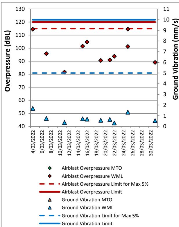
Figure 69: Warkworth Blast Monitoring Results - March 2022
