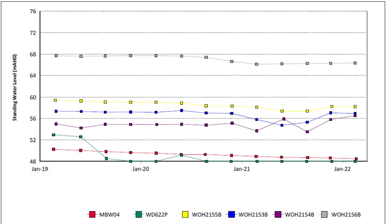
Figure 36: Wambo Seam Standing Water Level Trend – March 2022
