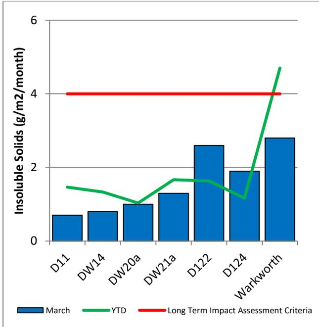
**Figure 4** displays insoluble solids results from depositional dust gauges during the reporting period compared against the year-to-date average and the annual impact assessment criteria.
