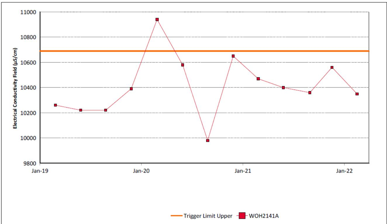
Figure 62: Whynot Seam Electrical Conductivity Field Trend - March 2022
