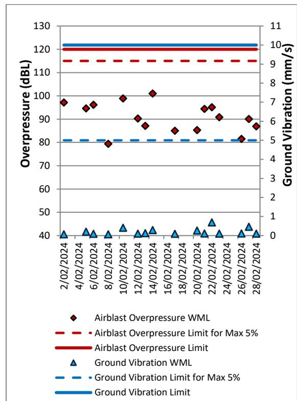
Figure 14: Warkworth Blast Monitoring Results – February 2024
