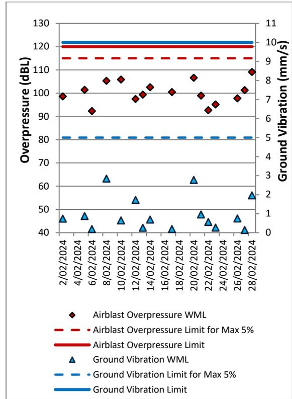
Figure 13: Wambo Road Blast Monitoring Results – February 2024
