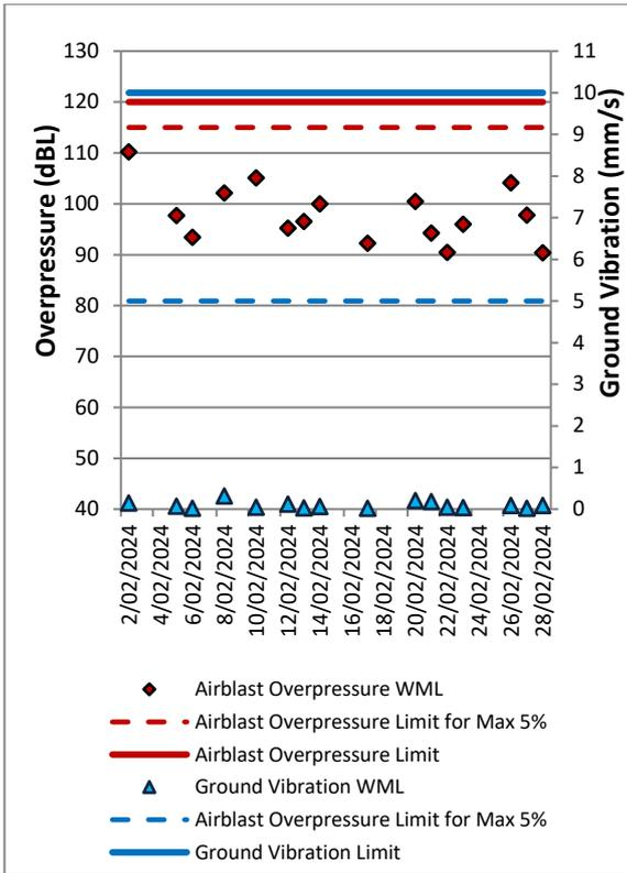
Figure 11: MTIE Blast Monitoring Results – February 2024
