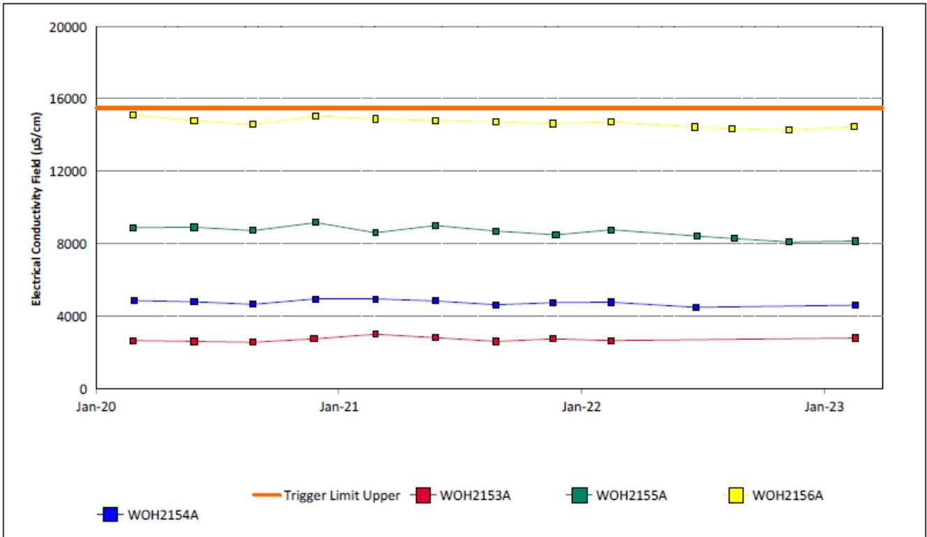
Figure 25: Redbank Seam Electrical Conductivity Field Trend – March 2023
